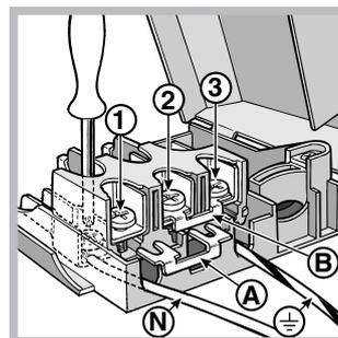
2. Position the connection support A (see figure) according to the connection diagram shown above. The terminal board is designed for single-phase 230 V connection: terminals 1, 2 and 3 are connected
