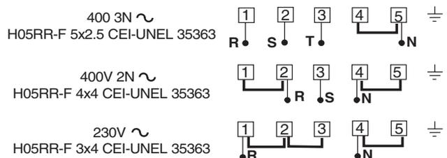
To install the power supply cable correctly:
