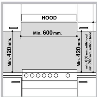
• If the cooker is installed underneath a wall cabinet, there must be a minimum distance of 420 mm between this cabinet and the top of the hob. This distance should be increased to 700 mm if the wall cabinets are flammable (see figure).
