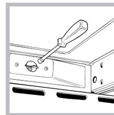
4. Unscrew the nozzle using a special nozzle socket spanner (see figure) or with a 7 mm socket spanner, and replace it with a new nozzle that is suited to the new type of gas (see *Burner and nozzle specifications table*).
