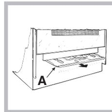
In gas cooker models, there is a sliding protection layer A that shields the lower compartment from the heat generated by the burner (see figure).
