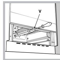
3. Remove the oven burner after unscrewing the screws V (see figure).
