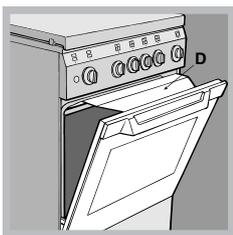
! When using the grill, leave the oven door ajar, positioning the deflector D between the door and the control panel (see figure) in order to prevent the knobs from overheating.
