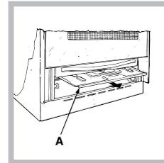
2. Slide out the protection panel A (see diagram).
