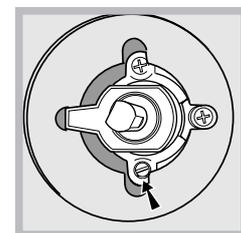
5. Turn the knob from the MAX position to the MIN position quickly or open and shut the oven door, making sure that the burner is not extinguished.
