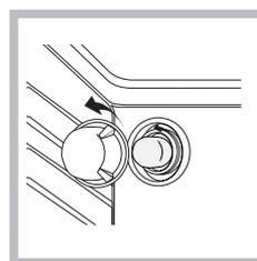
1. After disconnecting the oven from the electricity mains, remove the glass lid covering the lamp socket (see figure).
