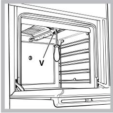
1. Remove the oven burner after loosening screw V (see figure).
