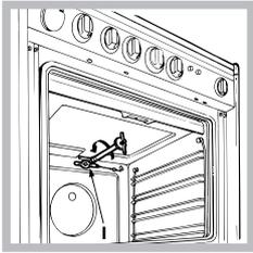
2. Unscrew the grill burner nozzle using a special nozzle socket spanner (see figure) or preferably with a 7 mm socket spanner, and replace it with a new nozzle that is suited to the new type of gas (see *Burner and nozzle specifications*
