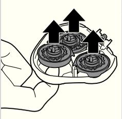
**5** Remove and clean one shaving head at a time. Each shaving head consists of a cutter and a guard.
